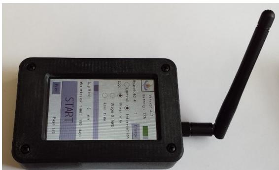
While our sensors can measure and log temperature like most SUMS loggers do, their real added value is that they can also directly detect and log whether the stove is being used or not. The EXACT sensors count cooking events and measure cooking time on-the-fly!
